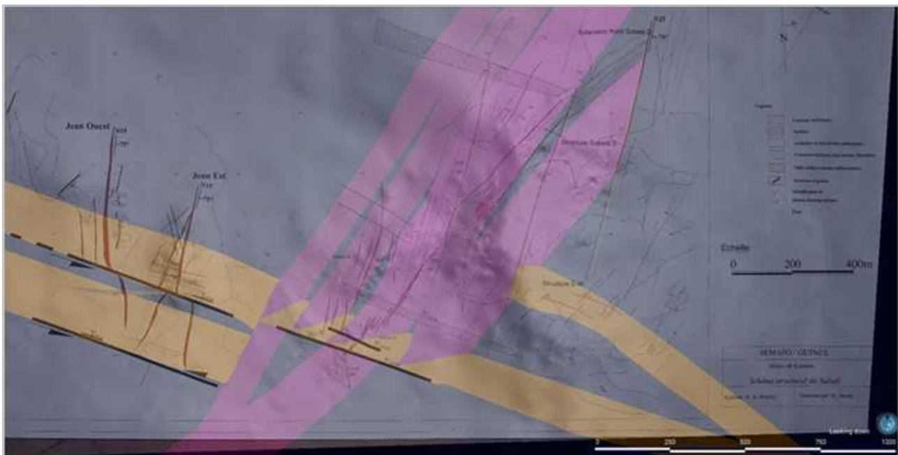
Figure 14.6 Historical SGA and Jean fault plan with digitized faults overlaid
