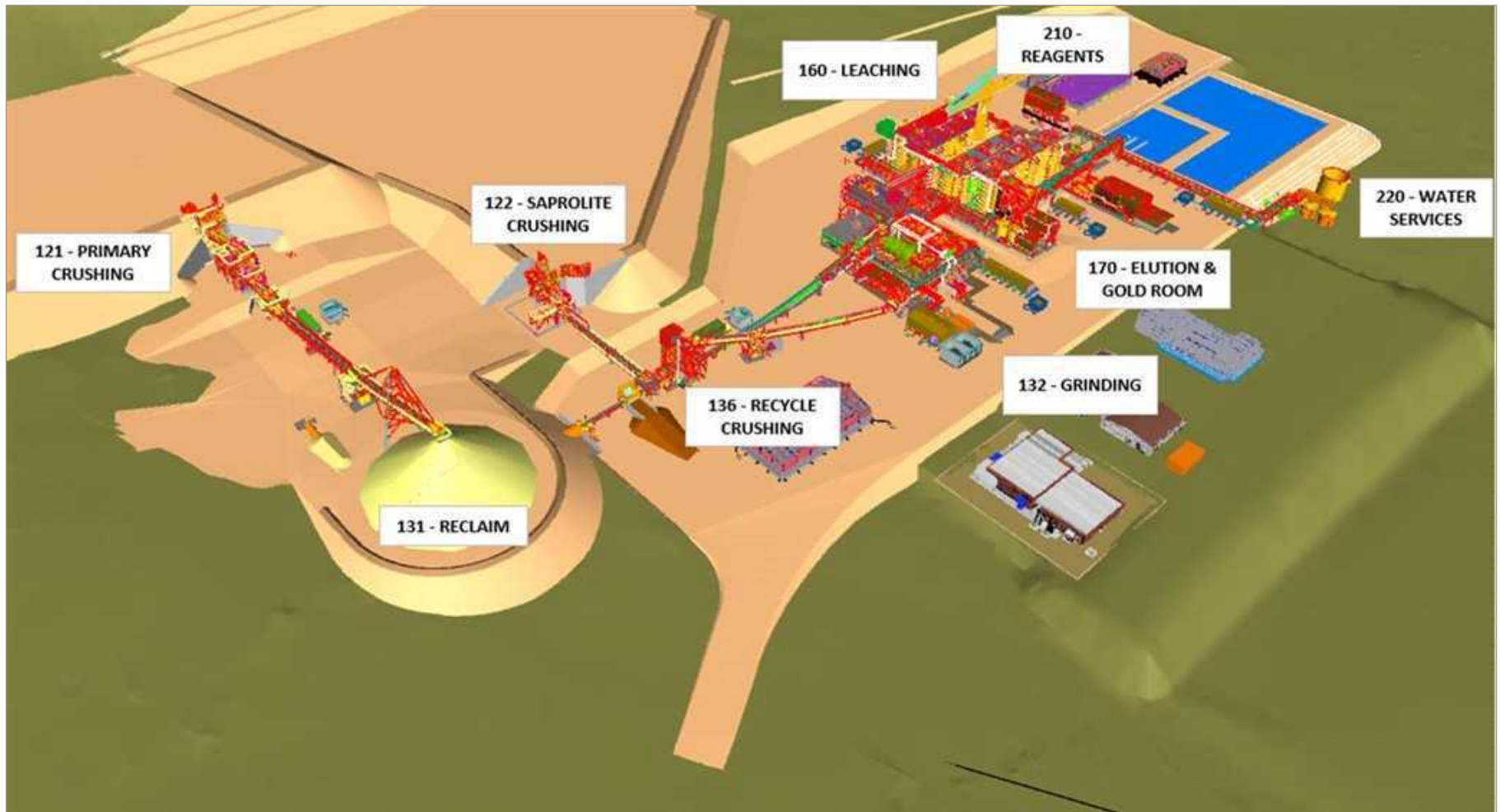
Figure 17.4 3D layout of the processing plant
